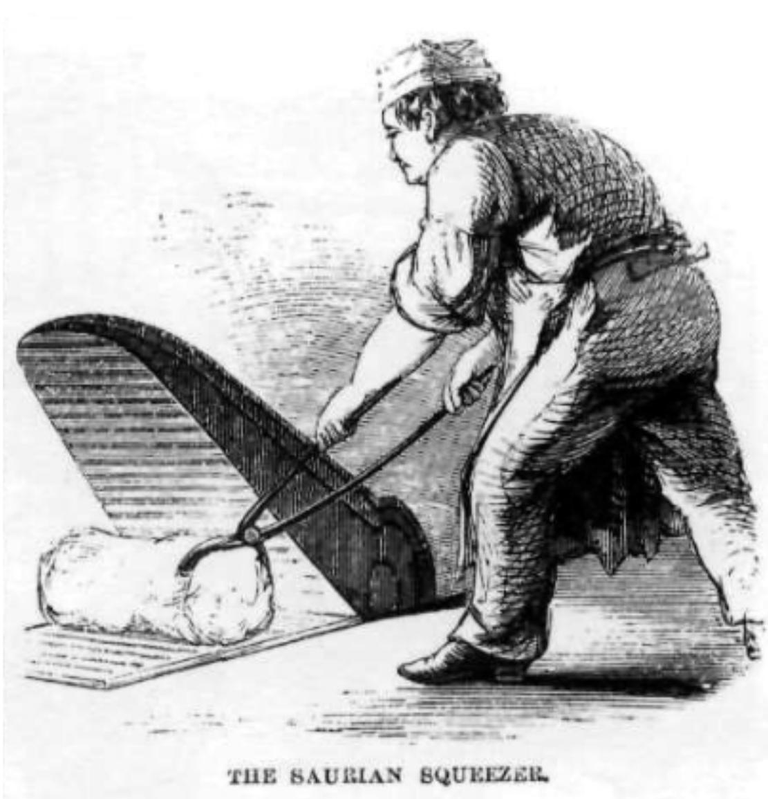
Figure 35. Drawing depicting puddled iron being squeezed in the 1860 article “Among the Nail-Makers” in *Harper’s New Monthly Magazine*.<sup>35</sup>
